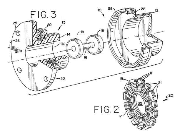
Figure 2 depicts stator 20 with conventional steel laminations 11 that form a magnetically inducible core 17 having a plurality of poles 21. *Id.* at 5:6–9. Wire windings 15 on core 17 serve as conductors, which induce or otherwise create magnetic fields in core 17 when electrical current is conducted through the conductors. *Id.* at 5:6–12.
